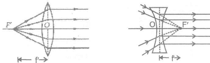
**Figure : Ray diagram showing First principal focus**
