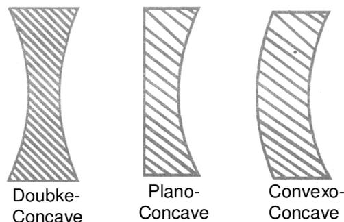
Figure : Different types of concave lens
