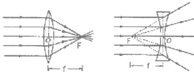
**Figure : Ray diagram showing second principal focus**
