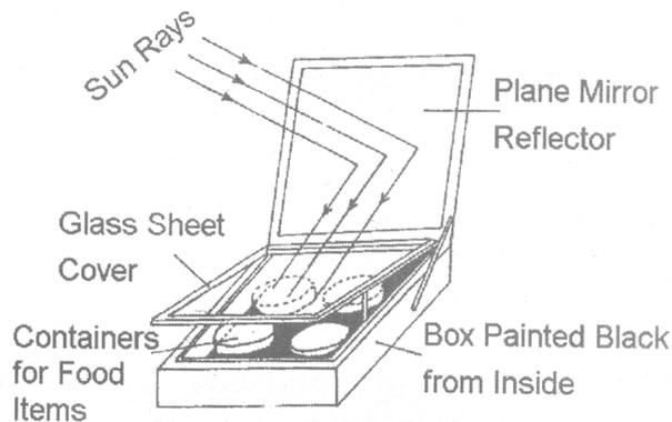
Solar cooker is a device used for cooking food with the help of solar energy. A box is made of a non - conducting material like plastic or fiber glass and painted black from inside is used for making the solar cooker.
