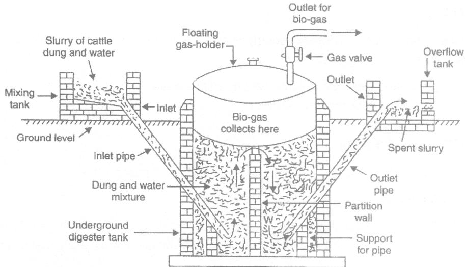
**Floating gas holder type biogas plant**
