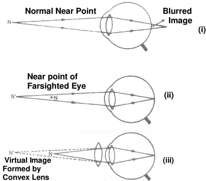
Figure : Correction of far sightedness by convex lens
