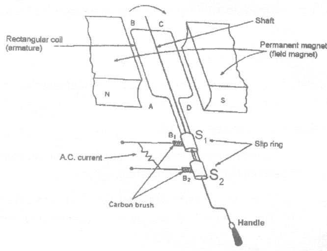
After every half revolution, each side of the generator coil starts moving in the opposite direction in the magnetic field. The side of the coil which was initially moving upwards, after half revolution, it starts moving downwards. Due to the change in the direction of motion of the two sides of the coil in the magnetic field every half revolution, the direction of current produced in them also changes after every half revolution.
