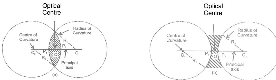
Figure : Characteristics of convex and concave lenses
